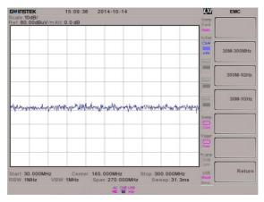
The GSP-9300 spectrum analyzer has a near field to far field conversion function that can be used when used in conjunction with these Field Sensors. When the Correction soft-key is selected, noise in the near field can be converted to radiated field strength in the far field accordingly. This can this be used to determine whether the test product will be able to comply with the 3M far field test.
